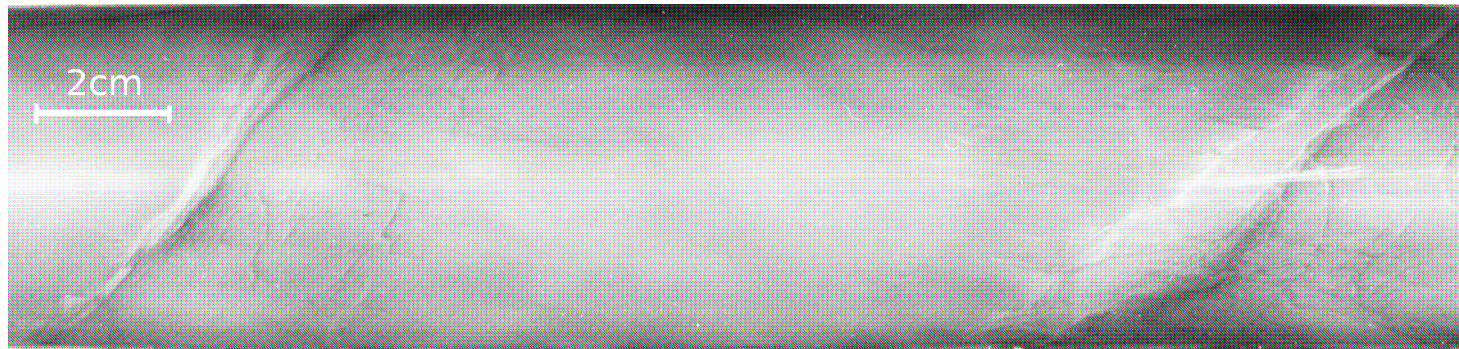
Experimental soot traces for CH 4 + 2O 2 mixture at P 0 = 50mbar.
